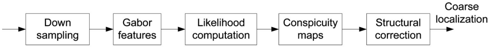
FIG 1. – Coarse landmark localization starts with computation of Gabor wavelets on downsampled images. Conspicuity maps for each landmark are computed by summing the likelihoods under mixtures of factor analyzers models. The most conspicuous locations are sent to the structural analysis subsystem for correction.
