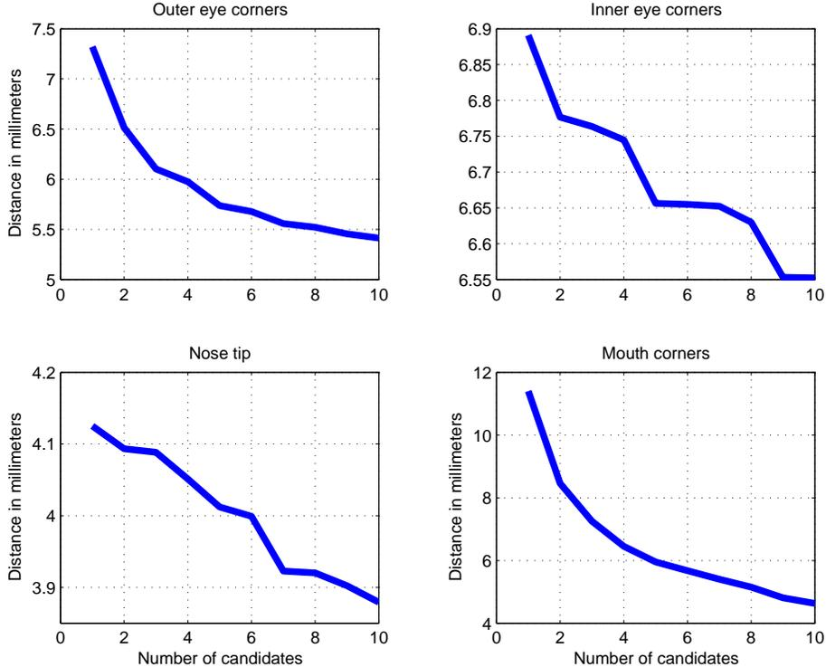
**Figure 1.** Accuracy of the automatic landmarking method, as indicated by average distance to true landmark in millimeters.
