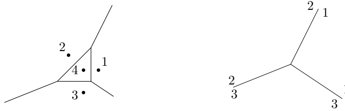
Figure 6: The Voronoi diagram of the points q_1(t), q_2(t), q_3(t) and q_4(t) for small positive t and at t = 0 .
