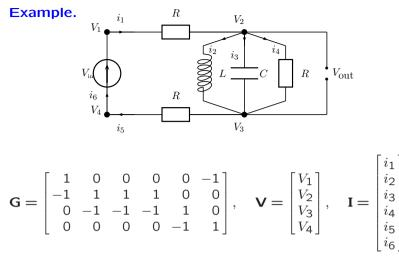
The size of the incidence matrix is  $k \times n$ , where k is the number of vertices and n the number of edges, that is, of electronic components. k = 4 and n = 6 in the present example.  $n \approx 5 \, 10^8$  in Intels dual-core i5.
