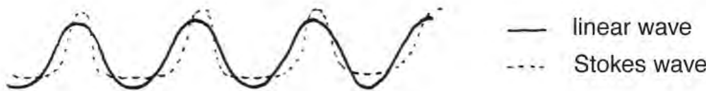
Figure 4.5: Profiles of a linear wave and of a Stokes wave, i.e., the sea surface elevation at a function of coordinate x at a fixed time. The waves travel from left to right.
