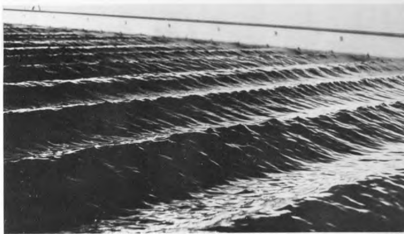
Figure 1.3: Waves generated in a laboratory with a moderate steepness ( \sim amplitude/wavelength). From Van Dyke [1982].
