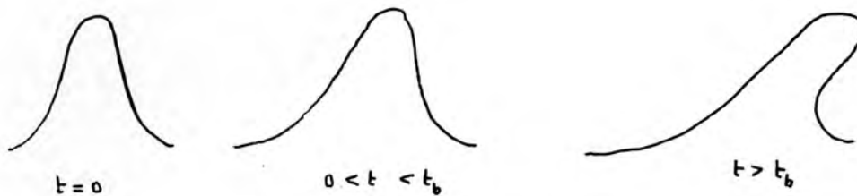
Figure 4.8: Profile of a gravity wave at different times computed from solving the nonlinear shallow water equations. After some time this wave breaks.
