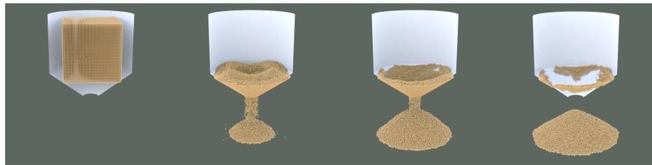
(b) Friction coefficient  $C_f = 2$
