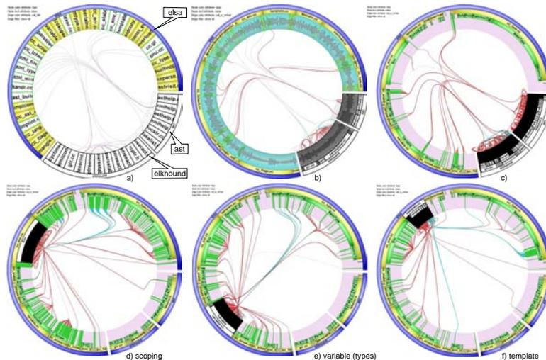
**Fig. 5.** OINK framework: multilevel visualization of calls on the level of files (a), classes (b), and functions (c); Main semantic analysis subsystems: the scoping environment (d), variables (e), and template analysis code (f). Selected subsystems are shown in black
