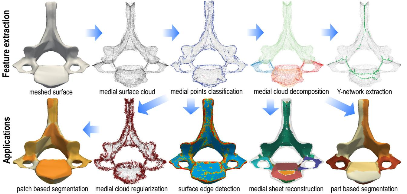
Fig. 1. Refined skeletal features computed from medial point clouds (top row) and subsequently enabled applications (bottom row).
