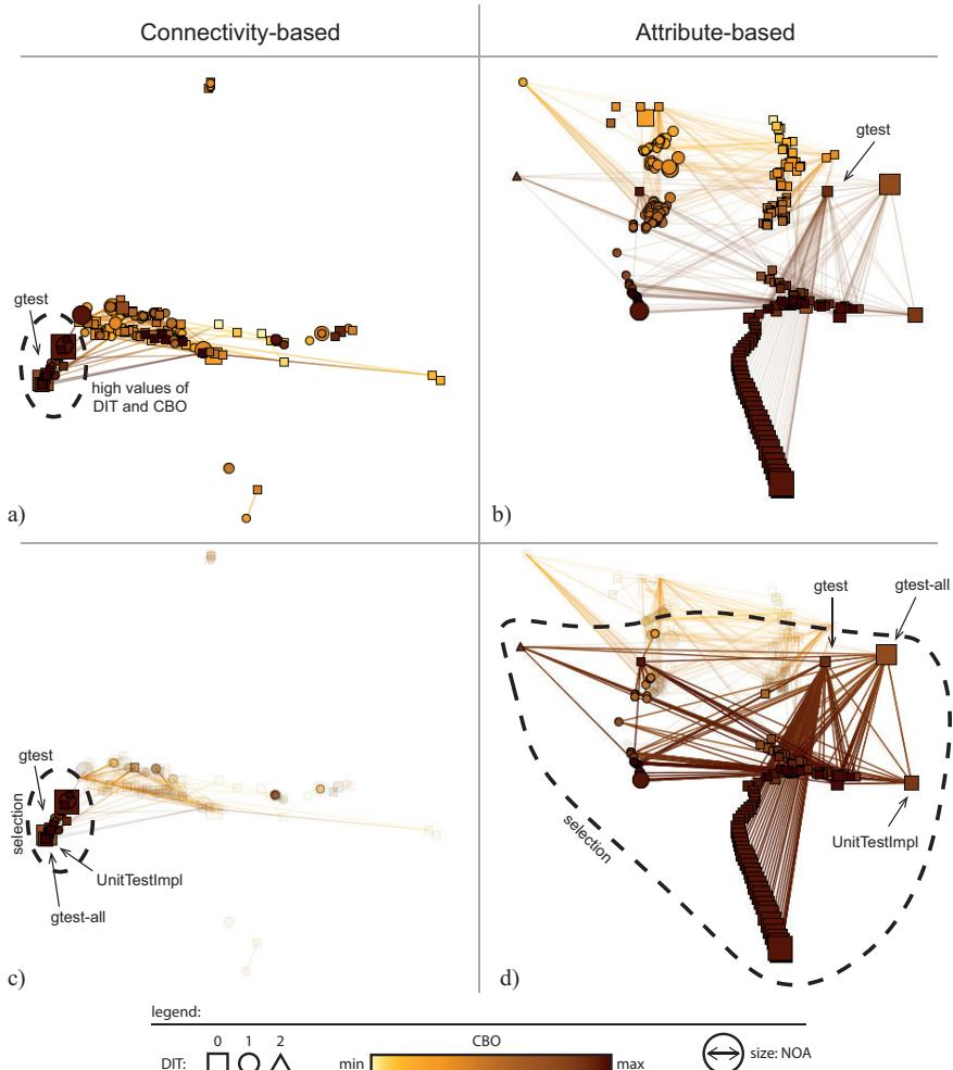
Figure 7.16: Projections of the *caffe* dataset, using the LSP projection technique, with attribute values encoded by node glyph sizes and colors. (a,c) Projection based on the shortest-path distance matrix only; (b,d) Projection based on the attribute values only. Bottom row (b,d) focuses the visualization on two selections of nodes, and thereby renders nodes outside these selections as half-transparent.
