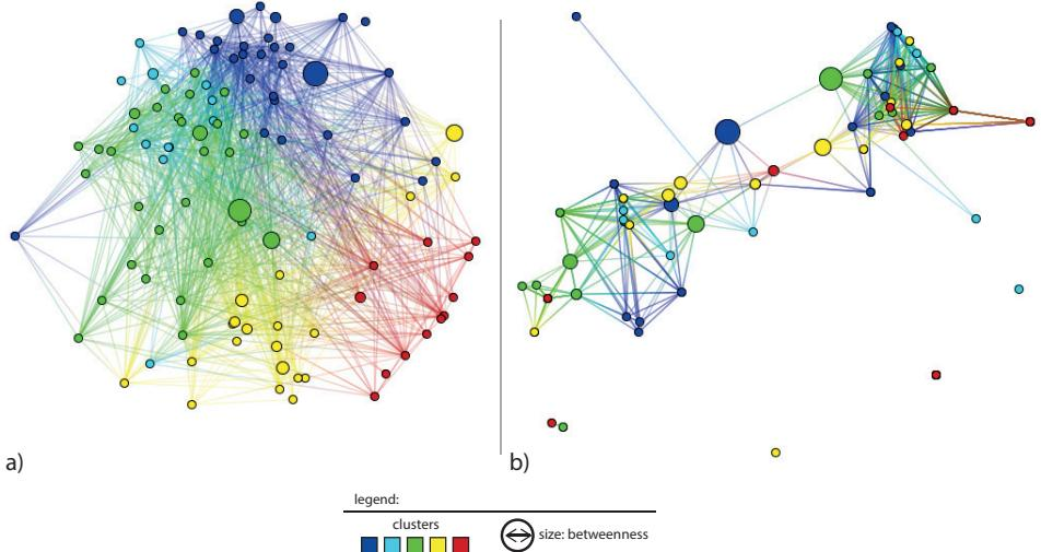
Figure 7.5: Two IDMAP projections of the *VisBrazil-Papers* dataset. (a) Projection using only the VSM node attributes. (b) Projection using only the shortest-path distance matrix encoding connectivity.
