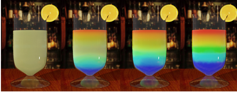
Figure 4.12: A fully mixed cocktail with phase separation due to the lack of interphase momentum.
