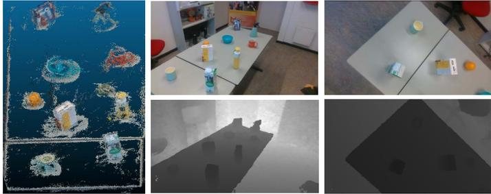
FIGURE 4.6: *The point cloud of the table2 dataset and examples of color-and-depth image pairs.*
