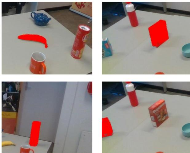
FIGURE 6.1: Visualization of estimated poses by our method. Each 3D model is projected to the image plane with the estimated 6D pose.
