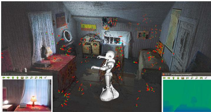
FIGURE 4.1: Snapshots from *PreSim* showing a robot moving in an indoor environment: the left subwindow is the synthesized color image and the right subwindow is the depth image.
