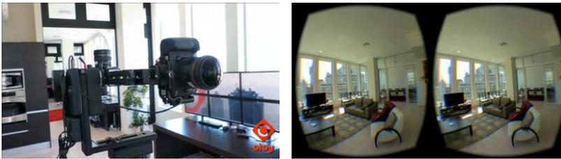
FIGURE 2.6: *The capture system for spherical light field and an example of synthesized images [DDB<sup>+</sup>15].*
