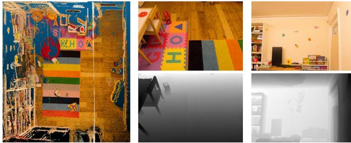
FIGURE 4.9: *The point cloud of the playroom dataset and examples of color-and-depth image pairs.*
