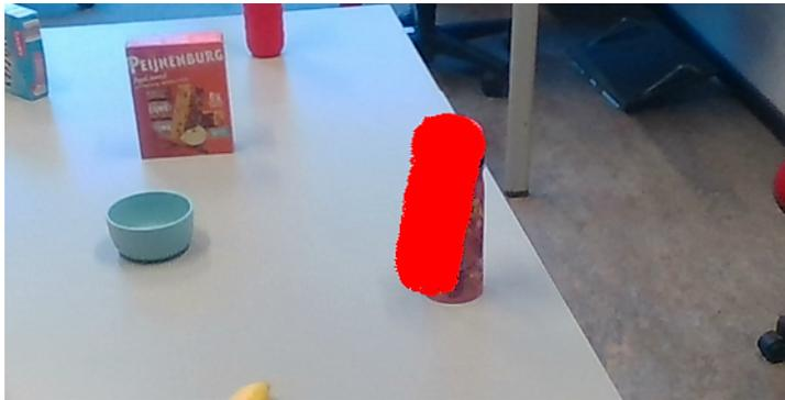
FIGURE 6.14: *The typical limitations of our approach: the estimated pose for the reflective object is not accurate, as the object projected by the predicted pose does not completely overlap onto the ground truth object. This is because it is hard to extract reliable features from reflective objects, which are used to estimate the pose.*
