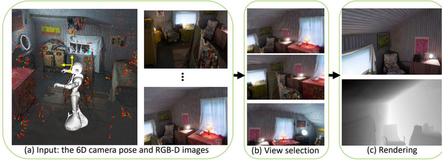
FIGURE 4.4: *The view synthesis pipeline including input, view selection and rendering. The input are RGB-D images and the 6D pose (red line shows positions of all the input image and yellow lines shows the 6D pose of the camera).*
