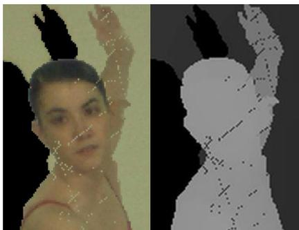
FIGURE 3.7: Problems caused by 3D warping in the synthesized image.
