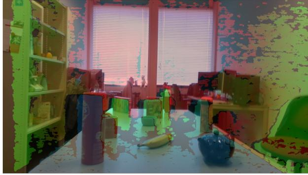
FIGURE 5.8: *Misalignment of color-and-depth image pairs. The images are generated when the distance between the object and camera is near, showing large misalignment.*
