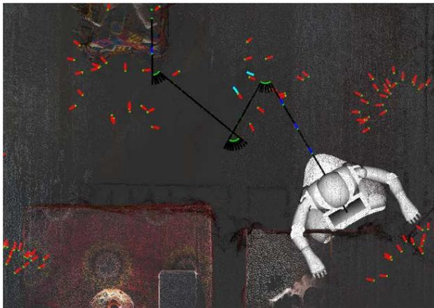
FIGURE 4.16: *The demonstrator model and its trajectory. Green points and red lines are positions and view directions of input views, light blue points and small blue lines are real-time positions and view directions of the virtual camera and the long line is the whole trajectory of the virtual camera.*
