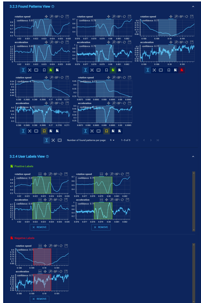
Fig. S49: Review Labels (File 2) . The user provided the labels shown in the figure for the second data file. To show the originating found patterns, we have included the Found Patterns View in the screenshot. Basically, the user marked the two true positives as positive labels and the top false positive as a negative label.
