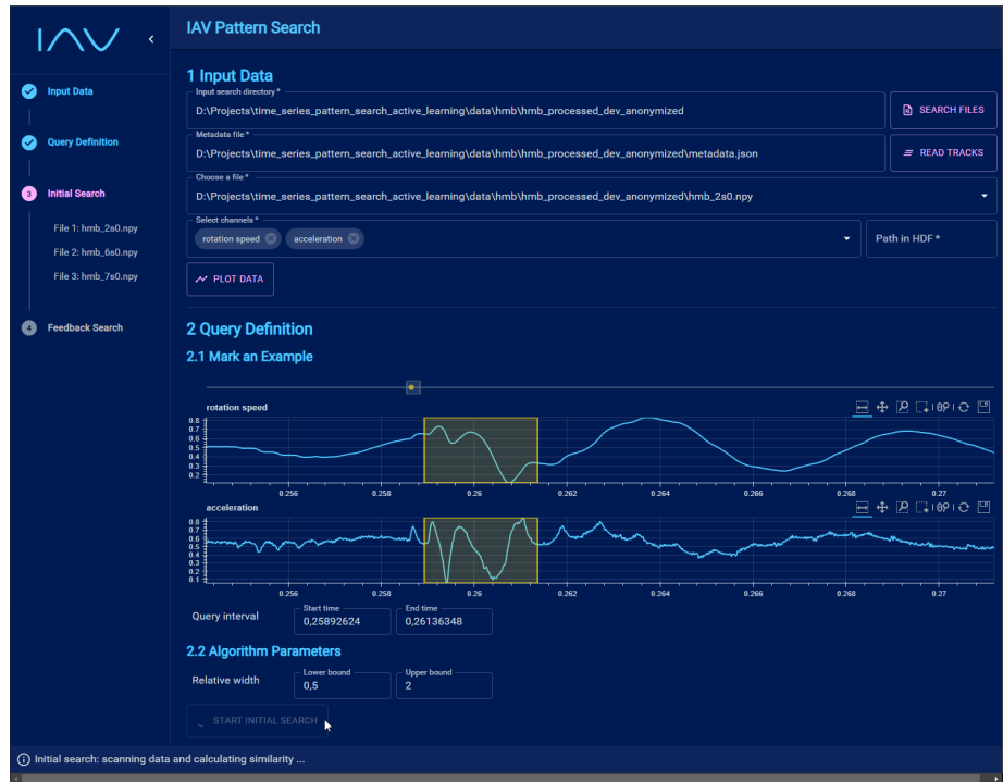
Fig.S42: Start Initial Search. The user clicked the button “Start Initial Search”, to run the quick-and-dirty rule-based initial search. The status bar reported on the processing status of the backend (computing similarity profiles, conducting dimensionality reduction for the scatter plot, calculating pairwise similarity between found patterns for the force graph, etc.)
