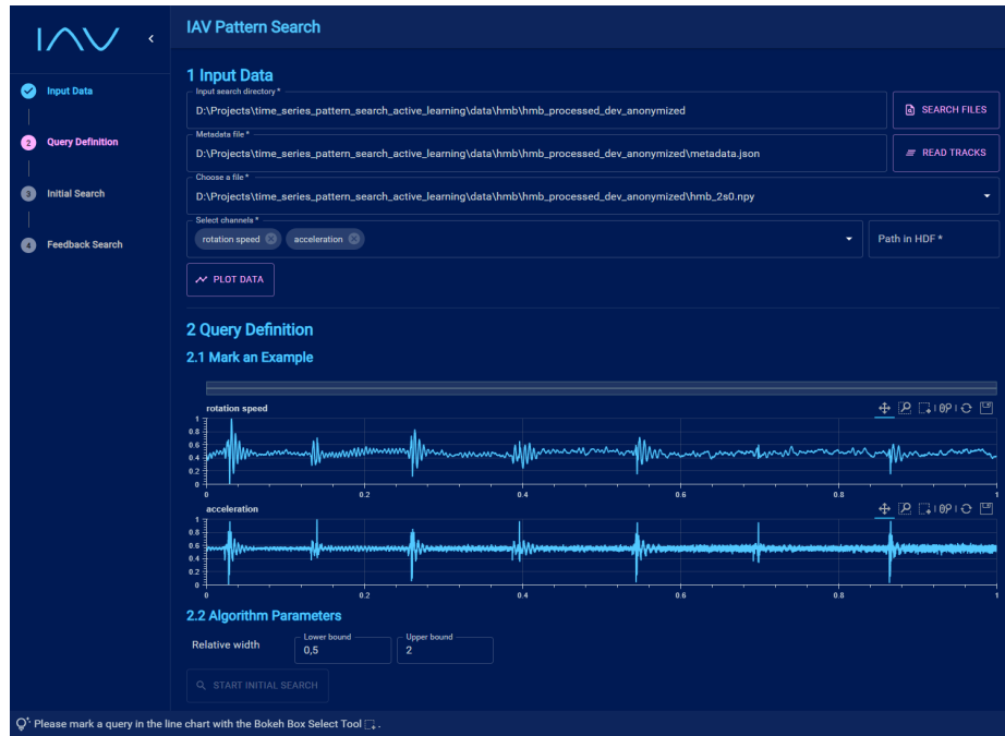
Fig.S40: Inspect Data. After clicking the button “Plot Data”, the selected channels in the chosen data file were plotted for inspection. The selected two channels roughly correspond to the engine rotational speed and acceleration. They were extracted by our engineers based on domain-specific signal processing techniques. We can see the harshness, or periods where the signals vibrate with high amplitudes, in the data. They occurred during transitions between half-engine operation and full-engine operation in a variable displacement engine. Because there are two types of transitions, namely, from half-engine to full-engine and vice versa, there are also two types of events. The transition from full-engine to half-engine looks more interesting because the harshness is more severe.
