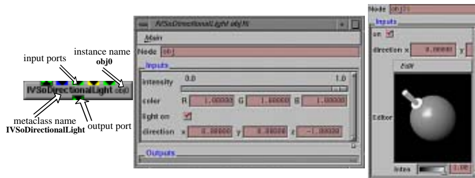
Figure 3. Left: Metaclass icon. The ports' graphical signs encode C++ type, by value/by reference and other attributes. Right: metaclass GUIs
