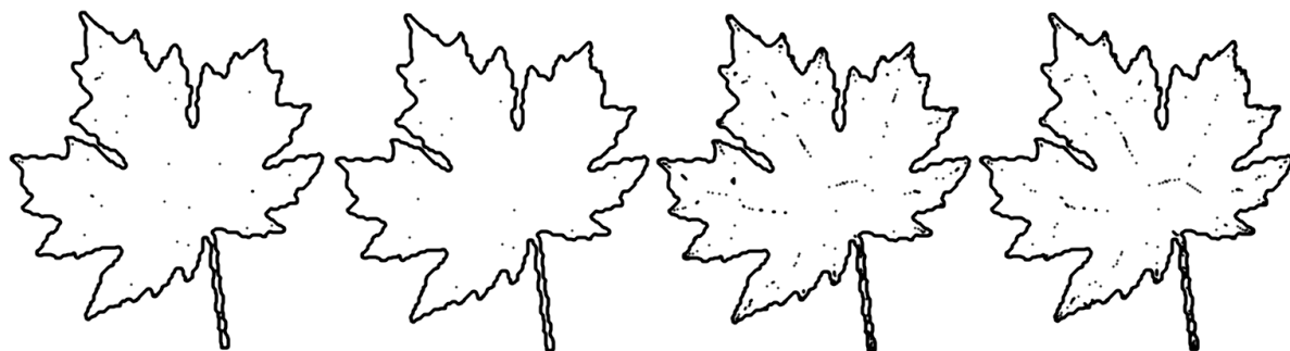
Figure 8: Locations of origin errors for the leaf image, \epsilon = \sqrt{2} . From left to right: FMTFT8, \epsilon VDT8, GTFT8, and ETFT8. The boundary and erroneous pixels are thickened for better display.
