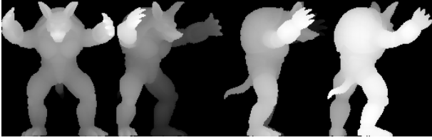
Fig. 4. The Z-buffers of the first four selected views in case of synthetic scanning.
