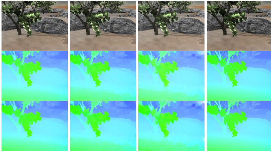
**Fig. 3.** Visual comparison on the Gaussian noise added Grove2 sequence [5]. **From Top to Bottom:** Grove2 sequences, flow results of WMF, flow results of PatchWMF. **From Left to Right:** flow with added Gaussian noise  $\sigma_n = 10$ ,  $\sigma_n = 20$ ,  $\sigma_n = 30$ , and the ground truth flows.
