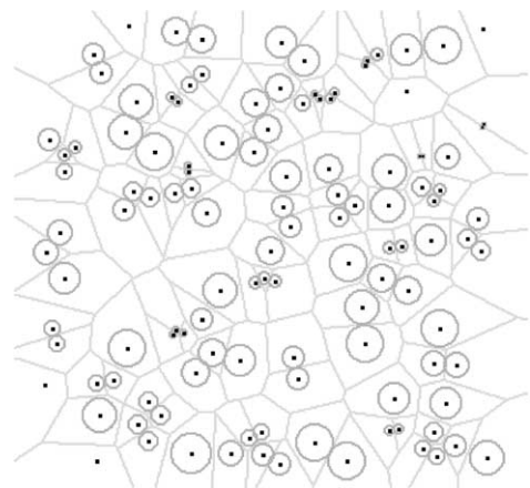
Fig. 7. Stienen model of a Poisson point process in E^2 . Two nuclei may touch at their common cell boundary iff the two are nearest-neighbours, but not all nearest neighbour balls do, due to asymmetry. Observe that none of the radical centres can be covered.
