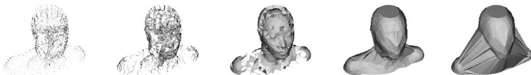
Fig. 1. Example of an evolving zero-weight \alpha -complex of a bust. Left: a small \alpha -value, yielding a complex that is little more than just the point set with a few singular edges, developing into right: high \alpha -value, yielding an overly fat complex obscuring all the fine details of the face and the next that almost evolved into the convex hull (data set by Silicon Graphics, 2780 points).
