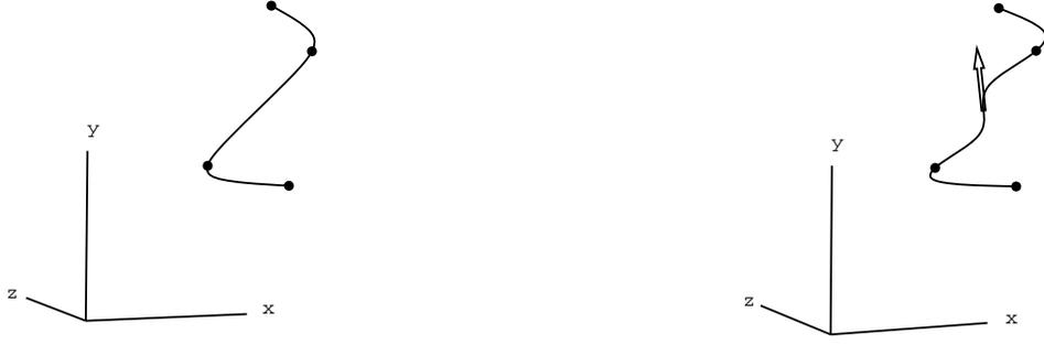
Figure 1: Left: minimal energy curve with point interpolation constraints. Right: with additional tangent constraint.
