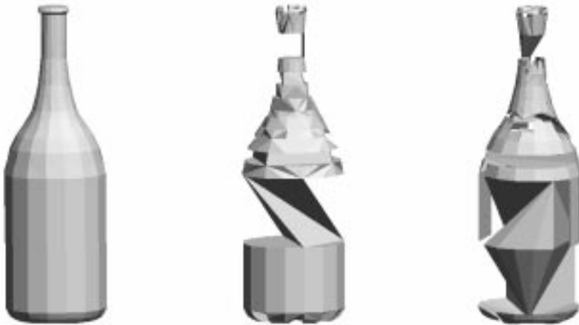
Figure 9: Comparing three methods on a set of vertices from a bottle's surface. Left: \gamma -indicator method. Middle: minimal area change method. Right: Voronoi skeleton method.
