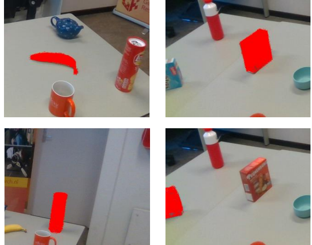
Fig. 1: Visualization of estimated poses by our method. Each 3D model is projected to the image plane with the estimated 6D pose.
