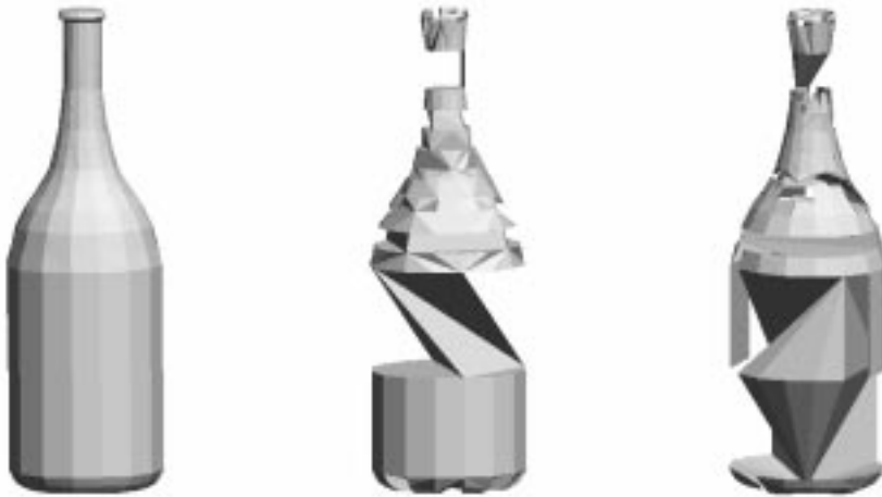
Figure 5.10. Comparing three methods on a set of vertices from a bottle's surface. Left: \gamma -indicator method. Middle: minimal area change method. Right: Voronoi Skeleton method.
