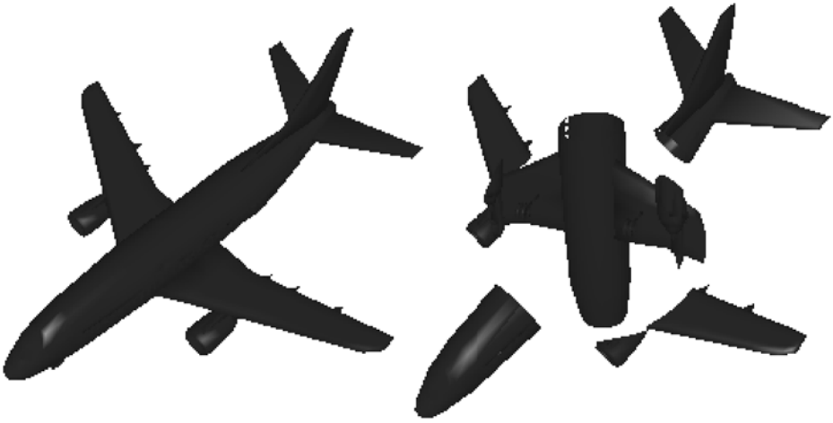
Fig. 6 Spherical harmonics do not distinguish models that differ by a rotation of an interior part [61]
