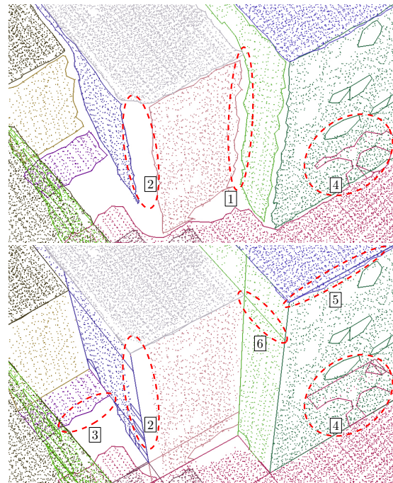
Figure 11: The \alpha -shapes (top) and guided \alpha -shapes (bottom) of part of a LiDAR data set, with interesting regions marked.
