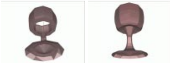
Figure 9: the effect of improper weight sets for the goblet \alpha -complex model. Left: the negative stem-to-cup weight zone is too large. By the time the increasing \alpha can override the negative weight, the entire zone will be bridged at once (observe the singular edges). Right: the negative weight zone is too small; the points at the inside bottom of the cup are able to connect, whereas the points from stem-to-cup are not. Compare to figure 7.
