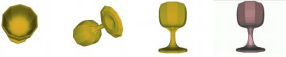
Figure 7: leftmost three figures show the zero-weight \alpha -complex of a goblet data set ( n = 520 ). Close examination shows extraneous faces in the stem-to-cup transition. Applying a non-zero weight set (figure 8) lifts this defect. The final result is shown at the right (data set obtained from GEOMVIEW DISTRIBUTION).
