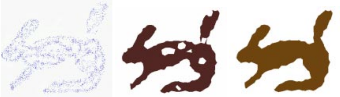
Figure 10: rabbit-like animal, free-form shaped by spraying “coloured” weight on a 400 \times 400 regular rectangular canvas. RGB-colours are translated to normalised weight w \in [-1..1] : w = \pm \frac{1}{2} \bar{R} \pm \frac{1}{3} \bar{G} \pm \frac{1}{6} \bar{B} , where \bar{R}, \bar{G} and \bar{B} denote normalised colour components (gray-levels) for red (heavy) weight, green (medium) weight and blue (light) weight, resp. Left: blue-coloured S (observe sparsely sampled spots). Centre: \alpha -complex of the blue-mask rabbit. Right: rabbit overlaid with a green weight mask covering the sparse locations; the 6 holes of the central figure have now vanished.
