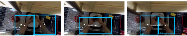
Fig. 5. A double hand detection finds its way into the right hand track.
