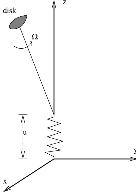
Figure 4: Rotor with diskmass  $M$ , elastically mounted with axial ( $u$ ) and lateral directions.
