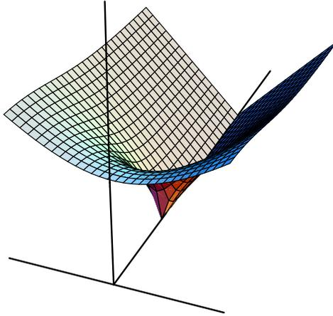
Figure 3: The critical surface in  $(\mu_+, \mu_-, \delta_+)$  space for eq. (24).  $\mu_+ = \mu_1 + \mu_2$ ,  $\mu_- = \mu_1 - \mu_2$ ,  $\delta_+ = \delta_1 + \delta_2$ . Only the part  $\mu_+ > 0$  and  $\delta_+ > 0$  is shown. The parameters  $\delta_1, \delta_2$  control the detuning of the frequencies, the parameters  $\mu_1, \mu_2$  the damping of the oscillators (vertical direction). The base of the umbrella lies along the  $\delta_+$ -axis.
