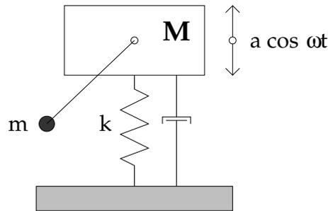
Figure 5: Two coupled oscillators with vertical oscillations as Primary System and parametric excitation of the coupled pendulum (Secondary System).
