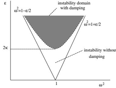
Figure 2: First order approximation of instability domains without and with damping for eq. (20) near  $\omega^2 = 1$ .
