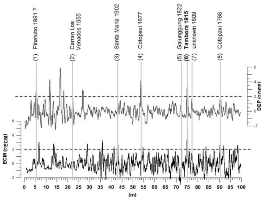
**Fig. 2.** DEP (upper plot) and ECM (lower plot) conductivity record of ice core S100. Peaks assigned to known volcanic events (volcano and the year of the eruption are marked) and used for dating purposes are numbered. The data are filtered and normalized, and the threshold is established at  $2\sigma$  (dashed line).
