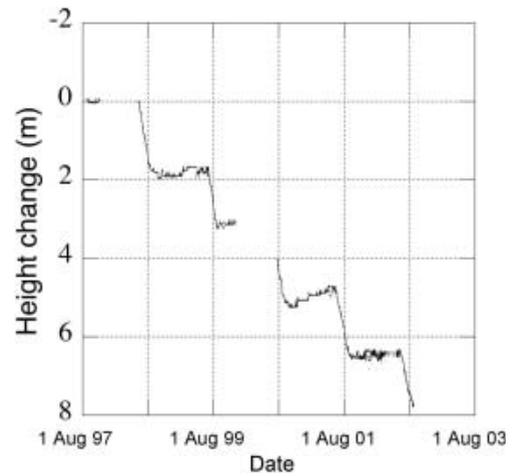
**Fig. 6.** Cumulative change of elevation as measured with the sonic height ranger at site 6 over 5 years, with 1 August 1997 chosen as reference level. Data gaps are estimated based on stake readings.
